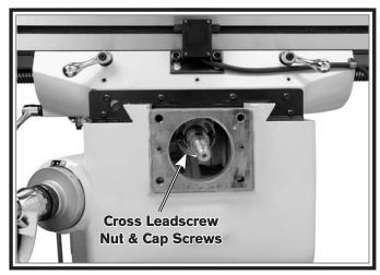
Figure 64. Cross leadscrew nut and cap screws.
